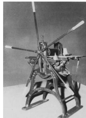
Hand-operated “Spider” press with flat plate, which was used by the BEP to print the bicolored stamps
